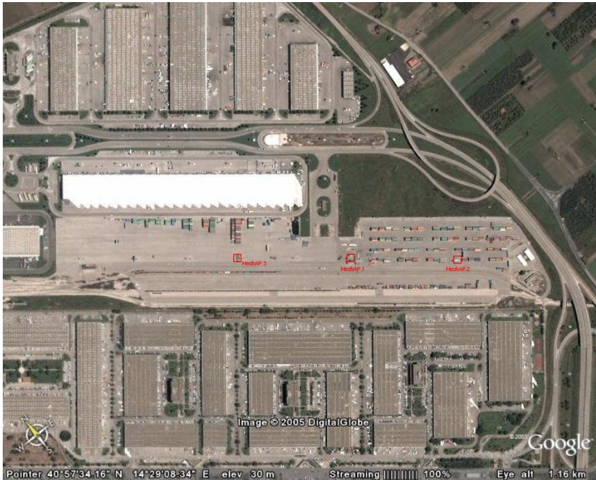
Figure 7.2: Aerial view of the Nola interport with the disposition on fixed nodes mounted on top of the light towers, corresponding to the red squares.
