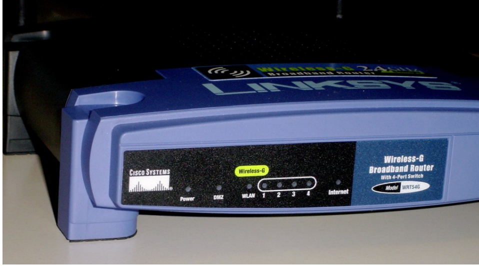
Figure 4.2: Front visual of the WRT54g wireless router, the lights used to check the router status are visible. The LED marked as DMZ is used to give feedback on the boot-up of the operating system, as it is turned off when the boot sequence is terminated and it is ready to start routing operations.
