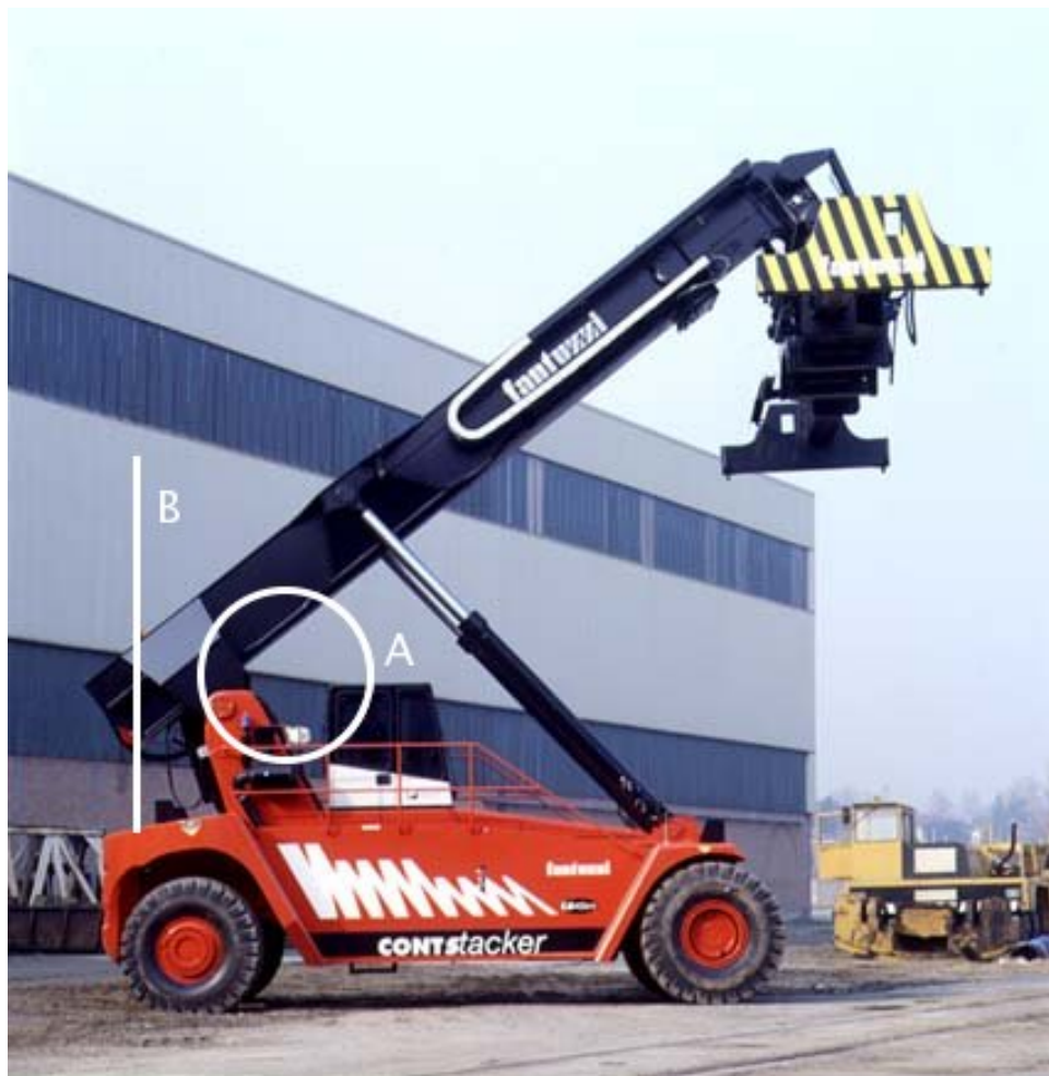
Figure 7.3: Positioning of the MeshAp on the stacker: the letter A shows the position of the hardware, while B is the position of the antenna on top of a pole.
